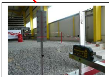
Measurement Point Chassis Warpage
